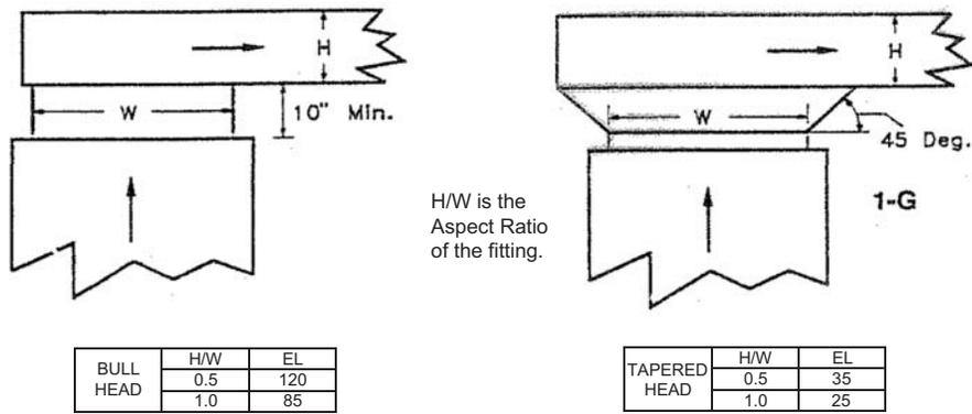
The H/W Height/Width ratio must be calculated to determine EL equivalent length.
