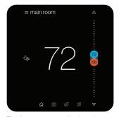
The **home screen** displays the current temperature, the system mode, a set-point adjustment slider, and icons leading to the other top-level screens.
