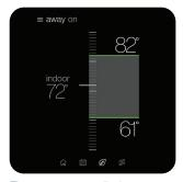
The **away screen** displays energy saving set-points. Away mode can be selected manually or entered automatically using geo-fencing in the Daikin *One* home app.
