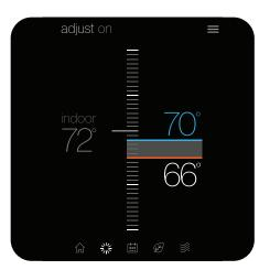
The **adjust screen** displays the current temperature on the left and set-points on the right. Change the set-points by dragging them or by turning the dial.
